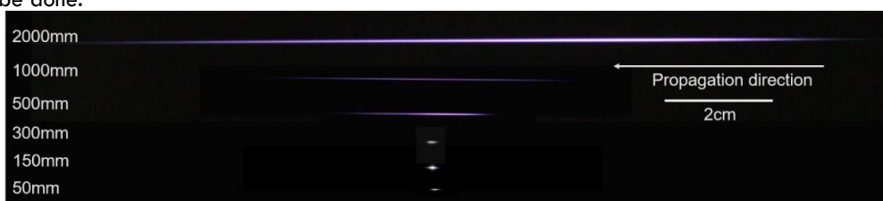
Figure 13. : Images of the filaments imaged using the DSLR Nikon t4i camera. Exposure and gain was adjusted to capture complete spatial extent of the filaments generated using the lens with focal length=50mm, 150mm, 300mm, 500mm, 1000mm and 2000mm.
